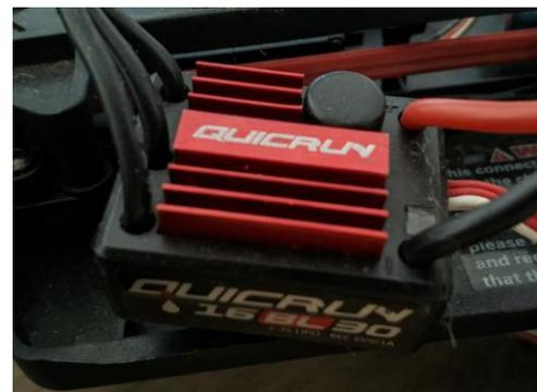
Gambar 6. *Electronic Speed Controller*.
